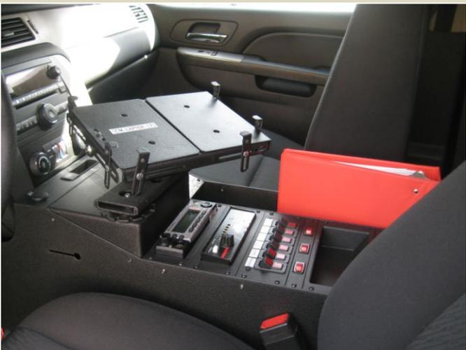
(Photo 3) Same console with “insert” computer mount. Uses 7” of sloped area otherwise used for equipment face plates. 13-23” available for faceplates (depending on which model). Shown with console-insert laptop mount.
